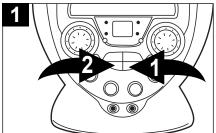
After you insert the disc into the CD player and the total number of tracks appear on the display, you may press either the Skip/Search (►►I) ① or (►►I) ② button to select a specific track for playback.
